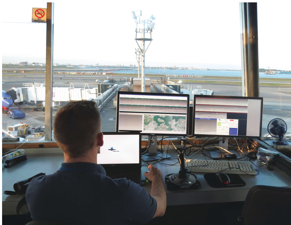
The Interceptor warns air traffic controllers of potential threats, and they can then modify flight paths or delay departures briefly to prevent flight paths from intersecting.
